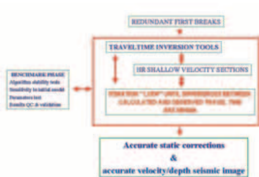
Fig. 6b. Near surface tomography processing flow.
