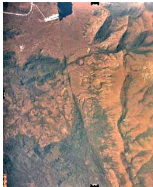
Fig. 3. Aerial photo of the Lake Edgar Fault, north up the page. A post-last-glaciation fan from the mountains to the east has planed and then been dissected by the last movement on the fault. Water ponded against the downstream face of Edgar Dam (off the top of the page) and the fault can be seen at the top of the photo. The prominent white east-west scarp is a former airstrip, the trench and exploration pits are a few hundred metres parallel to and south of the airstrip (see fig. 5).
