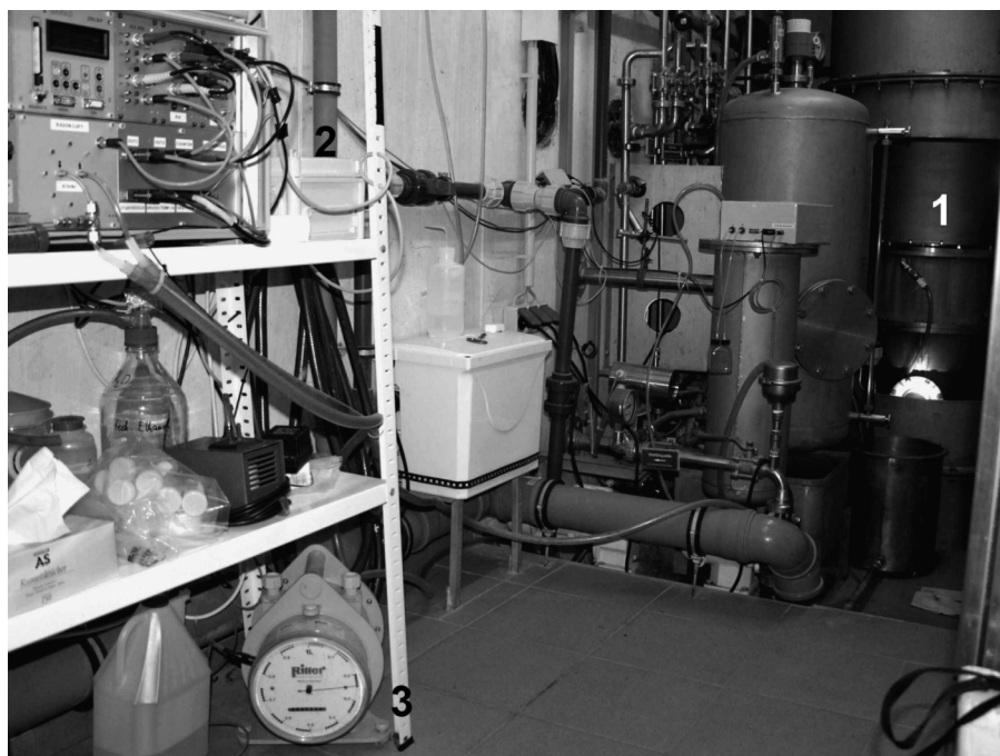
Fig. 3. 'Wetтинquelle' spring basement with spring capture (1), multiparameter station (2) and gas flow counter (3); technical details: see Koch et al. (2003).
