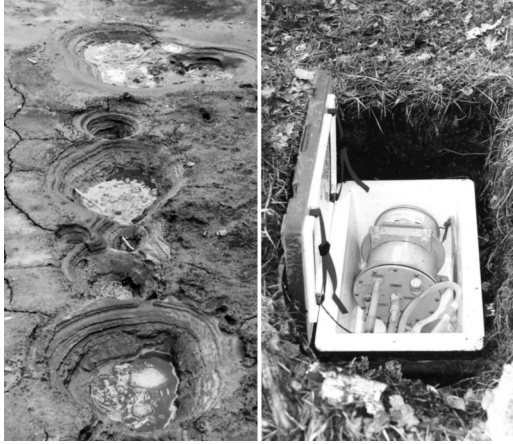
Fig. 4. Mofettes in the Nature Park Soos (CZ) and RITTER gas flow counter at the measuring mofette (right).
