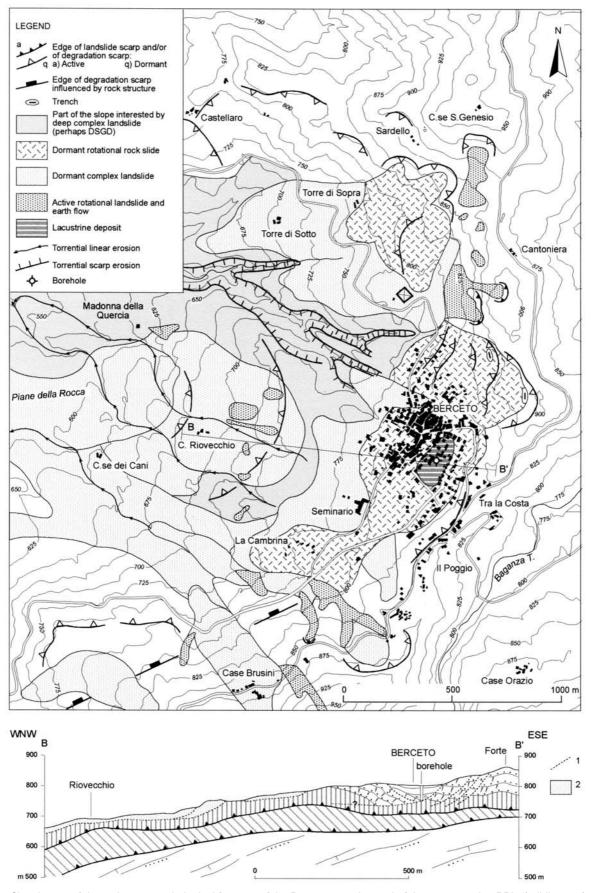
Fig. 3 - Sketch map of the main geomorphological features of the Berceto area. Legend of the cross-section BB': 1) sliding surface of landslide, 2) landslide body; for the geologic symbols used in it see the legend of Fig. 1.
