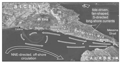
Fig. 3 - Overall seawater circulation of NE Sicily. S-directed, long-shore currents, due to Messina Strait, hydrodynamics interact with clockwise, offshore circulation of Ionian Sea.
