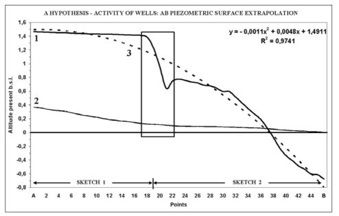
Fig. 6a - Real hydrogeological section and theoretical best – fitted on 2° degree equation extrapolation for **A** scenario. The rectangle represents the present Archaeological Park area. 1 = Past Piezometric Level; 2 = Present Piezometric Level; 3 = Past Extrapolation Level based on "Y" 2° degree equation.
