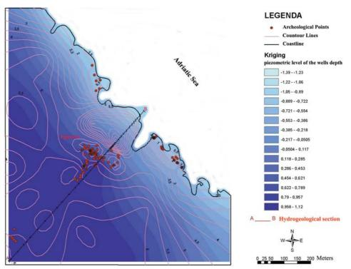
Fig. 5 - Piezometric surface restitution of Egnazia town, by means of ArcMap 8.3 GIS software, for B scenario.
