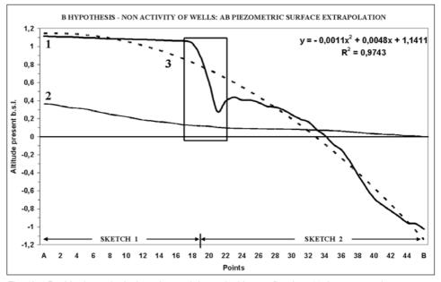
Fig. 6b - Real hydrogeological section and theoretical best – fitted on  $2^{\circ}$  degree equation extrapolation for **B** scenario. The rectangle represents the present Archaeological Park area. 1 = Past Piezometric Level; 2 = Present Piezometric Level; 3 = Past Extrapolation Level based on "Y"  $2^{\circ}$  degree equation.
