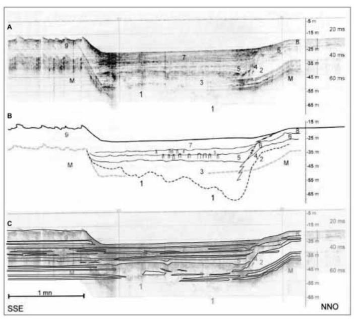
Fig. 2 - The seismic profile (A) located to the south of La Playa beach ridge (Fig.1) used by ORRU et al. (2004) to establish an unconformity between Holocene and Tyrrhenian deposits (B). Interlayering is evident in our interpretation (C).
