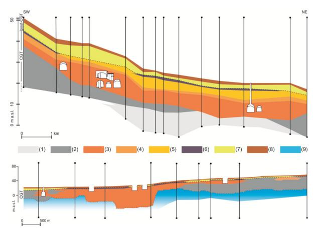
Fig. 2 - Geological cross-sections (tracks in Fig. 1): (1) *cinerite*,(2) grey tuff, (3) zeolitic yellow tuff, (4) pebble tuff, (5) incoherent facies of CGT, (6) paleosoil, (7) pyroclastic deposits younger than CGT, (8) soil, (9) pre-CGT deposits. Quarries and cavities are not to scale. Dotted line indicates the upper and lower limits of the CGT deposits.
