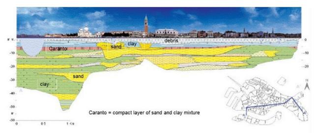
Fig. 2 - Subsoil geological setting of Venezia along a cross-section (after Zezza 2008).
