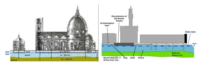
Fig. 1 - Schematic subsoil setting of the main historical buildings at Firenze.
