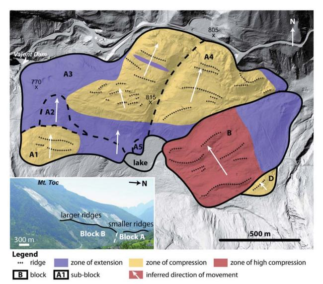
Fig. 4 - Morphostructural features of the Vajont Landslide deposits, showing zones of extension and compression, as well as blocks within the deposit. (Source: Wolter et al., 2015.)
