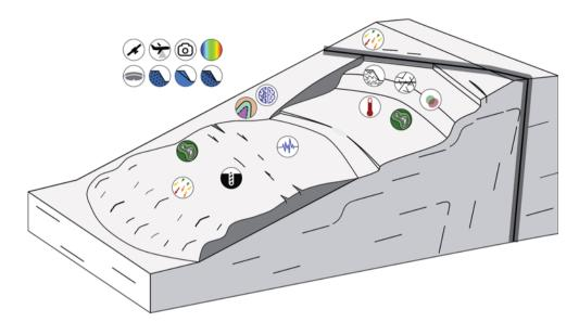
Fig. 1 - Structural features and controls (such as folds, fault zones, rock bridges, crown cracks, transverse cracks and ridges, and radial cracks) on landslides, with methods used to investigate them represented by icons. See Tab. 1 for legend of icons.
