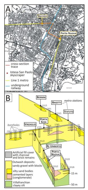
Fig. 15 - A) Main recent excavations in the subsoil of Turin: 1) subway (Line 1 of the Metro, 15 km); 2) underground railway pass (12 km); 3) Intesa Sanpaolo skyscraper. B) Cross section along the subway involving the variously cemented Dora Riparia River outwash sediments (modified from a Geodata sketch).
