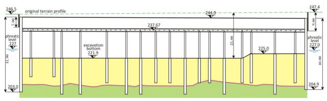
Fig. 16 - Cross section of the excavation of the Intesa Sanpaolo skyscraper (S in Fig. 14) essentially involving the outwash sandy gravelly sediments (yellow), with a boulder level, that lie on the silty Villafranchian succession (green). Altitude is referred as m a.s.l.
