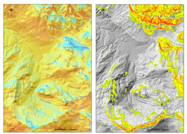
Fig.8 - Left: distribution of yearly global solar radiation (intensities increasing from dark blue to dark brown). Right: distribution of areas with slope angles above 30° (slope angles increasing from green to red).
