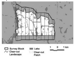
Fig. 3. Aerial survey plan for a clear-cut landscape. North-south transects are spaced 0.5 min of longitude (600 m) apart.
