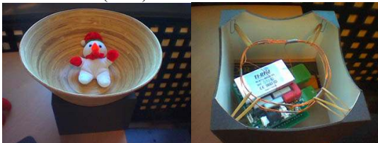
Figure 13: MediaTray for physical hypermedia interaction. The right picture shows the RFID tagreader in the bottom.
