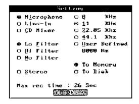
The Sound Blaster Pro card used in the study did not have a resolution option; those systems which permit audio capture at both 8 and 16 bit resolution will have one more option to set. In the present study 8 bit resolution was entirely adequate; 16 bit resolution provides for better audio fidelity, but for voice recordings. be they male or female, 8 bit resolution is entirely sufficient, and saves memory usage.
