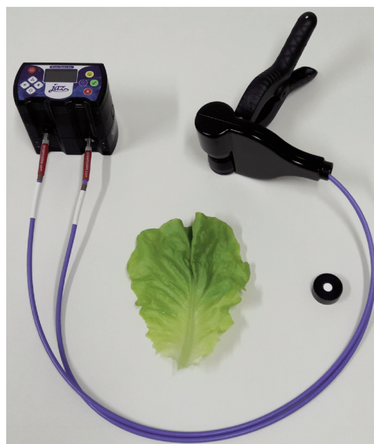
Fig. 1 - Hand-held spectrometer, clip probe, and diffuse reflectance standard used to collect reflected light from the lettuce leaves.
