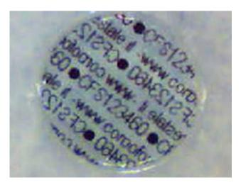
Fig. 1. Microdot disc of 0.5 mm in diameter.
