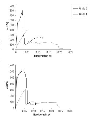
**FIGURE 3.** Typical real stress-Hencky strain curves for puncture test, above: transversely, degrees of maturity 4 and 5; below: longitudinally, degrees of maturity 4 and 5 of sweet passion fruit.
