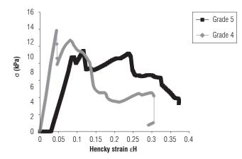
**FIGURE 2.** Typical real stress-Hencky strain curves for unidirectional compression test, longitudinally, degrees of maturity 4 and 5 of sweet passion fruit.
