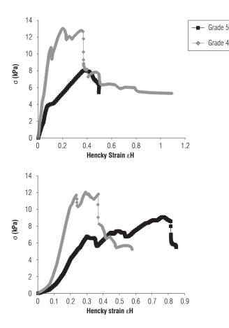
**FIGURE 1.** Typical real stress-Hencky strain curves for a unidirectional compression test, above: in the transversal direction, degrees of maturity 4 and 5 without *mallalon*; below: with *mallalon*, transversal direction, degrees of maturity 4 and 5 of sweet passion fruit.
