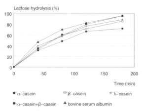
Fig. 4. Hydrolysis of lactose at 55°C in buffer B with added milk proteins . 7 ONPG units of enzyme activity were added per ml of buffer B.
