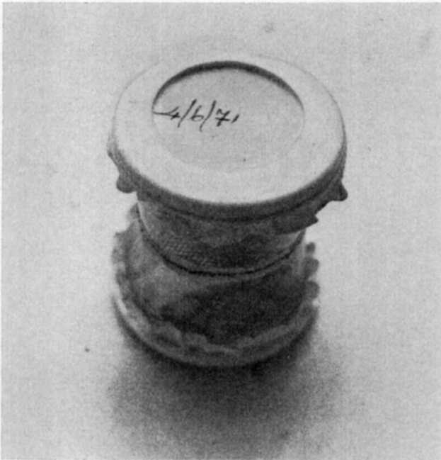
Fig. 1. A two chamber reproduction cage with filter paper between the snap-on lids and chambers. The net in between the chambers keeps adults in one chamber but nymphs can easily leave this chamber and enter the other.
