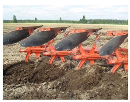
Suppl. Fig. 3. Skimmers installed on plough (between the mouldboards). This plough was used in experiment 1.
