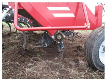
Suppl. Fig. 2. The working principle of Kvick-Finn cultivator: goosefoot tines loosen the soil and after that a PTO-driven rotor throws soil and weed roots into the air.
