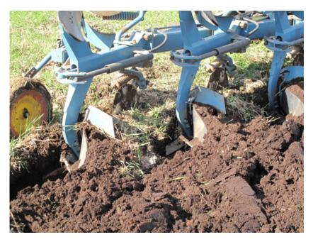
Suppl. Fig. 4. Trashboards installed on plough (above the mouldboards). This plough was used in experiment 1 and 2.
