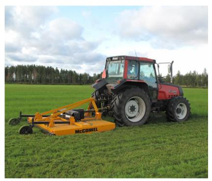
Suppl. Fig. 9. Horizontal rotary mower which was used in experiment 2 in the second year.
