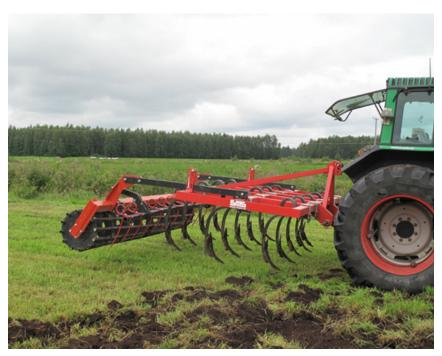
Suppl. Fig. 7. Tined cultivator with narrow blades was used in experiment 2 in the first year.
