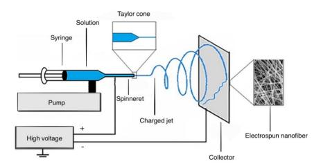
**Figure 2.** Electrospinning basic set-up design. Adapted with permission from Y. Li *et al.* Electrospinning in Tissue Engineering. In: A. Haider, S. Haider. Electrospinning: Material, Techniques, and Biomedical Applications p.117-139. Copyright (2016) IntechOpen [51].
