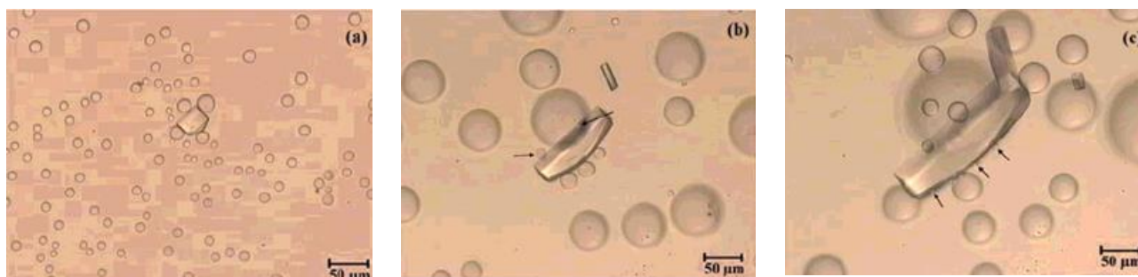
Figure 2. Time sequence of liquid-liquid phase boundary transformation to crystalline phase at 0, 12, and 22 h [26]. Reprinted with permission from S. Veessler, L. Lafferrère, E. Garcia, C. Hoff, Phase transitions in supersaturated drug solution. Org. Proc. Res. Dev. 7 (2003) 983-989. Copyright 2003 American Chemical Society.
