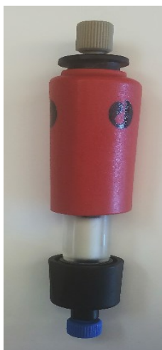
Figure 4. Cell membrane affinity chromatography column after packing IAM particles with the immobilized cell membrane fragments into a glass column
