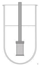
**Figure 1.** Schematic representation of the basket apparatus (Apparatus 1). Reprinted from ref. [3] with permission of Elsevier.
