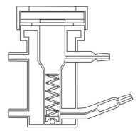
**Figure 4.** Schematic representation of the Franz-diffusion cell. Reprinted from ref. [3] with permission of Elsevier.
