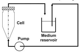
**Figure 3.** Schematic representation of the flow through cell. Reprinted from ref. [3] with permission of Elsevier.
