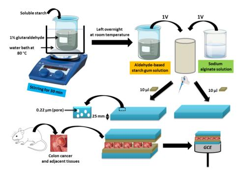
**Figure 3.** Schematic of the multilayer modification of GCE to study the detection kinetics of C and N nutrient receptors.
