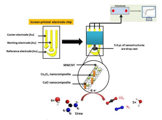
**Figure 5.** Schematic of CuO/Co<sub>3</sub>O<sub>4</sub>@MWCNTs preparation and electrochemical detection of urea. Based on the reference [121]
