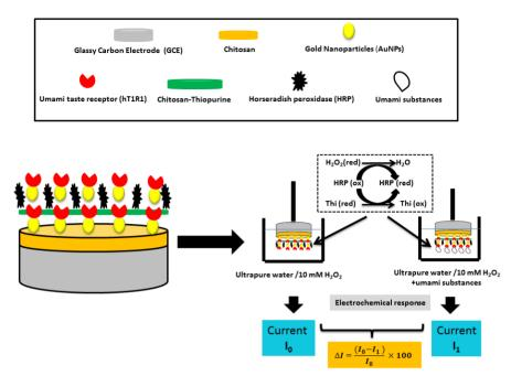
**Figure 2.** Schematic of the multilayer modification of the GCE to study the electrochemical response of the human umami taste receptor hT1R1 towards umami substances such as sodium glutamate, disodium inosinate and disodium guanylate. Carried out at the base of the reference [63] with an order License ID of 1346500-1
