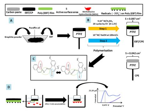
**Figure 1.** Schematic of A) EBT/CPE preparation, B) polymerisation steps of modified CPE, C) proposed mechanism of eriochrome black T (EBT) polymerisation and D) electrochemical detection of MDH by EBT/CPE. Carried out at the base of the reference [26] with an order License ID of 1346497-1
