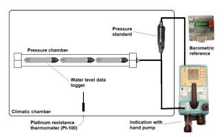
Figure 3: Calibration setup – scheme
