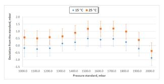
Figure 4: Deviation from the pressure standard at 15  $^{\circ}\mathrm{C}$  and 25  $^{\circ}\mathrm{C}$
