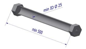
Figure 1: Pressure chamber
