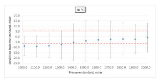
Figure 5: Deviation from the pressure standard at 10 °C
