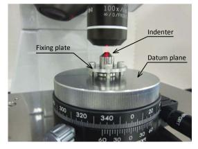
Figure 2. Setup of a Rockwell diamond indenter for the datum plane based profile measurement.
