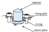
Figure 3. The detail of the sample fixture.
