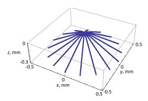
Figure 4. Measurement result of a Rockwell diamond indenter.
