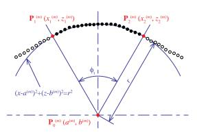
Figure 6. Extraction of the dataset of the spherical part from whole profile data corresponding to the central angle ft.
