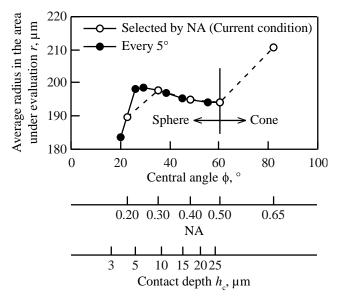
Figure 12. Average tip radius in the different evaluation area in the spherical part of indenter.
