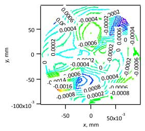
Figure 10. Deviation from the regression sphere of the spherical part of the indenter.
