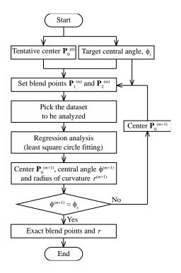
Figure 5. Flowchart for the determination of the tip radius  $R_a$  and the positions of blend points.
