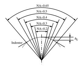
Figure 11. Evaluation of geometry of spherical part of indenter adopted by NMIJ.
