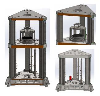
Figure 5: High Load Brinell Hardness Standard Machine
