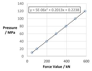
Figure 3: Fitting equation of tensioner
