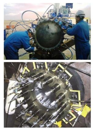
Figure 1: Application of stretcher in wind power and nuclear power industry
