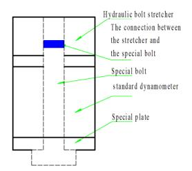
Figure 2: Schematic diagram of standard dynamometer calibration stretcher
