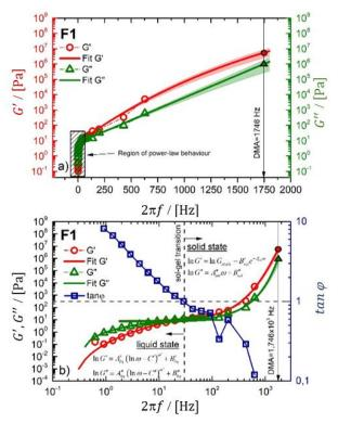
Figure 2: Fits of the storage modulus G', loss modulus G'', and damping factor  $\tan \varphi$  spectra against the oscillation frequency  $\omega$  ( $2\pi f$ ), according to equations (1) to (4), for the sample F1
