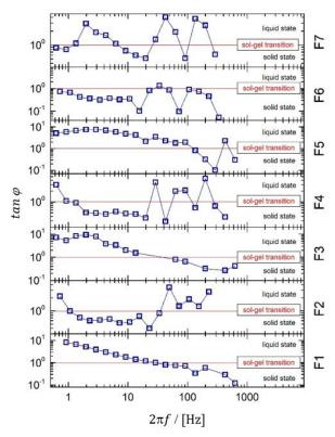
Figure 3: Damping factor  $\tan \varphi$  as a function of the oscillation frequency  $\omega (2\pi f)$  for the seven samples tested
