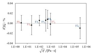
Figure 4: Weighted relative density mean values  $\delta' \overline{\rho_W}$  and respective uncertainties (vertical bars), obtained for the seven tested viscoelastic fluids (F#), against the squared root of dynamic viscosity ( $\sqrt{\eta'}$ ) of the fluids. Legend: S or L – sample at solid (S in red) or liquid (L in blue) state at the oscillation frequency produced in the oscillation-type density meter
