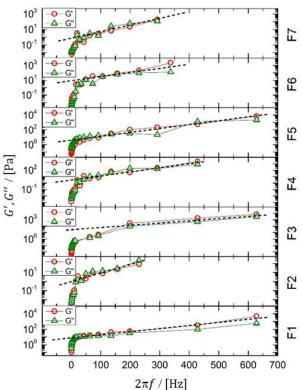
Figure 1: Storage G' and loss moduli G'' as a function of the oscillation frequency  $\omega$  (2 $\pi$ f). The black dashed line is a guide to the eye which depicts an exponential behaviour at higher frequencies
