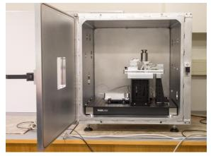
Figure 3: PB1 in a vacuum chamber. Visible on top of PB1 is a 1 kg mass standard.
