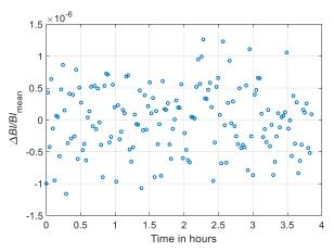
Figure 4: Repeated force mode measurement of a 1 kg mass standard. Each circle indicates a single ABBA cycle. The relative standard deviation for this measurement is  $0.6 \times 10^{-6}$ .
