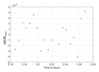
Figure 7: Repeated measurement of *Bl* in the velocity mode. The relative standard deviation is  $2.4 \times 10^{-6}$ . Each dot is the result of a 10 s measurement with a sampling rate of 10 kHz.
