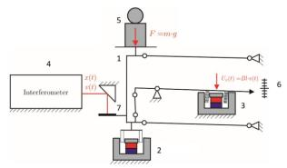
Figure 2: Schematic of PB1: 1-Load carrier, 2-External voice coil, 3-Internal voice coil, 4-Laser interferometer, 5-Weight, 6-Position sensitive device, 7-Mirror.
