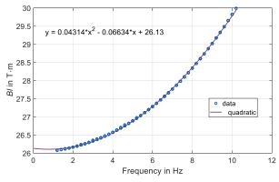
Figure 8: A measurement of the force factor *Bl* for different excitation frequencies.
