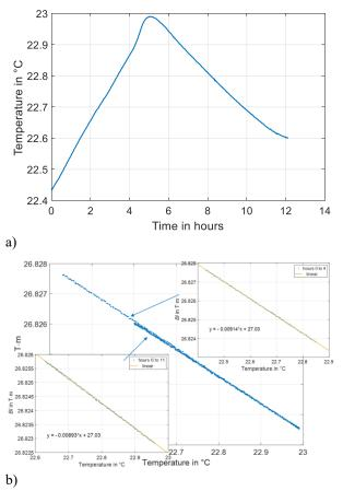
Figure 5: Measurement campaign of a 1 kg mass standard with PB1. The magnet shows a hysteresis. Depending whether the temperature is rising or falling with time, the temperature coefficient will be different by several per cent. a) Temperature measured in the magnet. b) The force factor Bl, measured during the campaign.
