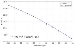
Figure 6: Measurement of the force factor Bl as a function of the coil position.
