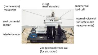
Figure 1: The setup of PB1 consists of a commercial load cell and an additional external voice coil attached to it. The motion in the velocity mode is measured with a laser interferometer. For automated weighing a mass lifter is used.
