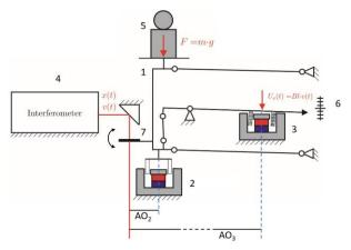
Figure 9: Explanation of the Abbe error in PB1: The external voice coil (2) has a smaller Abbe offset (AO2) than the internal voice coil (3), which is (AO3). The arrow at the mirror indicates that the mirror can tilt during up and down motion.
