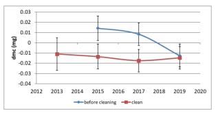
Figure 1: Typical calibration history  $(50 \text{ g}, \text{ E}_2)$  blue (upper) line shows deviation from nominal before cleaning; red (lower) line are values after cleaning. Uncertainty bars 95 %.
