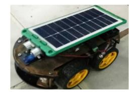
Figure 2. Assembled vehicle with the solar panel installed on the roof.
