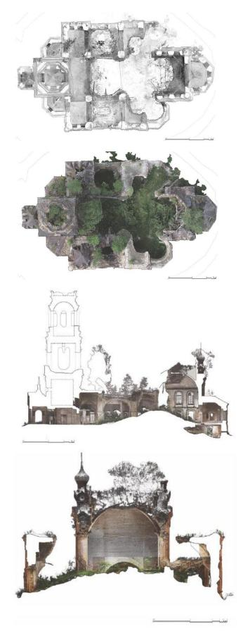
Figure 7. Drawings and elaborations for the 2D description of the main structural system of the church. The presence of noise data for elements such as the vegetation and collapsed ruins is highlighted.
