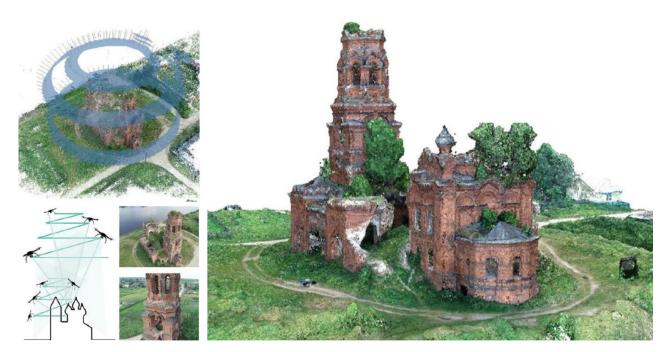
Figure 6. Morphometric database from the on-site photogrammetric UAV acquisition campaign: the photos were geo-referenced and aligned to define the main point cloud on the architectural complex and the surrounding landscape.
