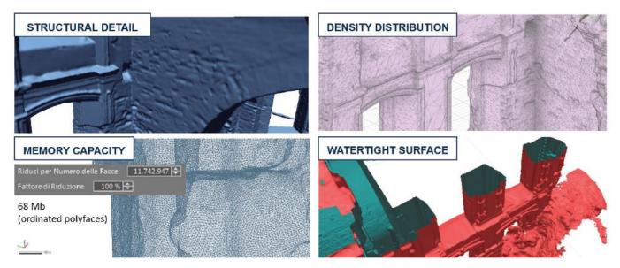
Figure 14. Properties of the final HD mesh model, which is suitable for compatible computing analysis in FEA workflows.
