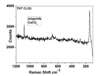
Figure 9. Raman spectrum of aragonite (CaCO<sub>3</sub>) on coin THT CLO3.
