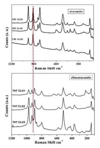
Figure 6. Raman spectra of copper trihydroxychlorides  $[Cu_2Cl(OH)_3]$  atacamite and clinoatacamite on the coins found at Tharros.
