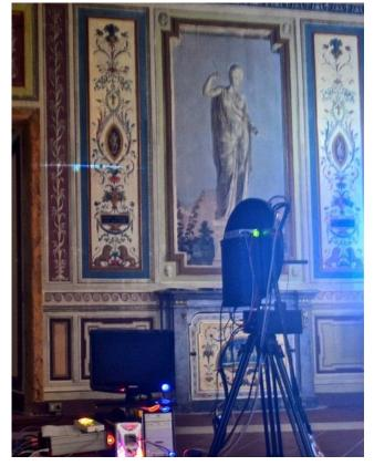
Figure 2. LIF system operating at the Bishop's Palace of Frascati. Laser beam line visible on the left wall.
