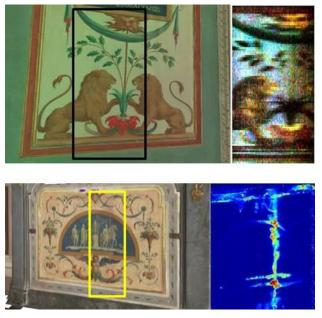
Figure 9. Top: RGB-ITR image with measured area in black line (left) and corresponding false colour LIF image (right).
