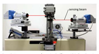
Figure 7. Measurement set-up for torsional stiffness with indicated sensing beams of autocollimators (red).
