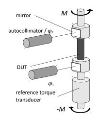
Figure 6. Torsional stiffness measurement set-up.
