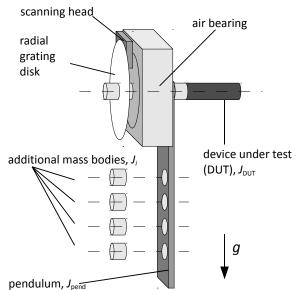
Figure 2. Pendulum for the measurement of the mass moment of inertia.
