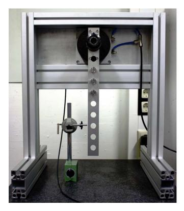
Figure 3. Measurement set-up for the determination of the mass moment of inertia, shown with three mounted mass bodies and mounted DUT.
