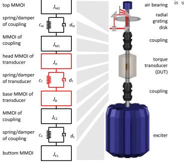
Figure 1. Measuring device and its model.
