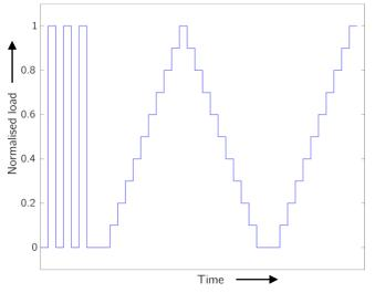
Figure 8. Load steps of the torsional stiffness measurement routine.
