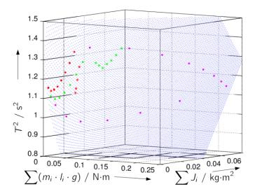
Figure 4. Measurement values for different auxiliary mass bodies mounted at different positions in the pendulum (red, green and magenta dots) and result of the bivariate regression (blue, dotted surface).
