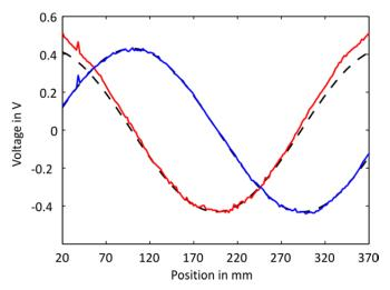
Figure 11. Demodulated output voltages  $U_{IA}$  (red) and  $U_{QA}$  (blue) of the two absolute receive channels compared to ideal sine and cosine (both black dashed) signals.
