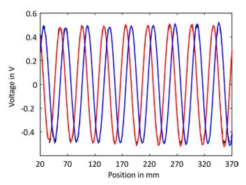
Figure 12. Demodulated output voltages  $U_{\rm IP}$  (red) and  $U_{\rm QP}$  (blue) of the two precise receive channels compared to ideal sine and cosine (both black dashed) signals.
