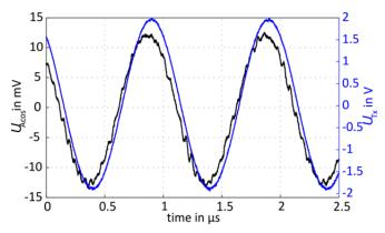
Figure 6. The measured coupling voltages on the absolute sine receive coil show voltage transients of 15 mV amplitude. The excitation voltage is approximately a 4 V peak–to–peak 1 MHz sine wave signal.
