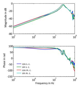
Figure 8. The Bode diagram shows the capacitive crosstalk behavior from the excitation winding to each of the four receive channels.
