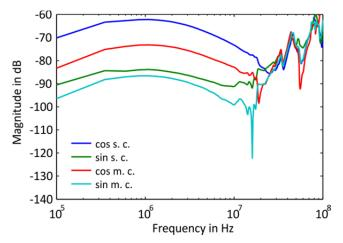
Figure 4. The plot shows the  $i_m/i_{Txr}$ ,  $m = \{Asin, Acos, Psin, Pcos\}$  behavior of the four receive windings due to direct inductive transmitter to receive coupling.  $i_{Asin}$  and  $i_{Acos}$  are the single cycle coil currents,  $i_{Psin}$  and  $i_{Pcos}$  are the multi-cycle coil currents and  $i_{Tx}$  is the excitation current.
