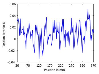
Figure 15. Position error of the multi-cycle coils along the measurement axis.
