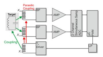
Figure 10. Functional block diagram of the signal condition electronic for the absolute or precise position receive coils.
