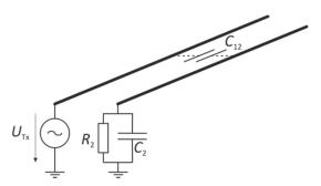
Figure 7. Simple model to describe the capacitive coupling between two parallel conductors.
