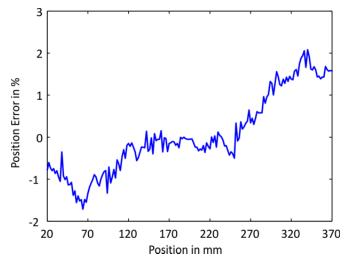
Figure 14. Position error of the absolute coils along the measurement axis.
