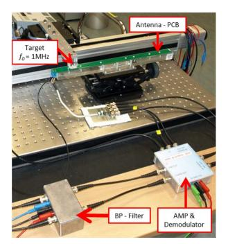
Figure 13. The picture shows a measurement setup of a high–frequency inductive position sensor for absolute linear position measurement. The used antenna design corresponds to the illustrated antenna PCB in Figure 1.
