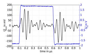
Figure 5. The measured coupling voltages on the absolute sine receive coil show voltage transients of 150 mV amplitude. The excitation voltage is approximately a 4 V peak–to–peak 1 MHz square wave signal.
