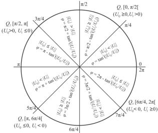
Figure 9. Arc-tan computation for measurement range  $[0, 2\pi x/l_A]$  [8].
