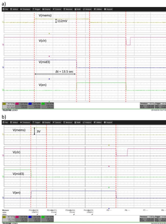
Figure 13. Results of the level shifter circuit for various input voltages: a) V_{in} = 112 \text{ mV} , b) V_{in} = 3 \text{ V}
