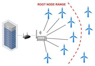
Figure 2. Traditional wireless sensor network.
