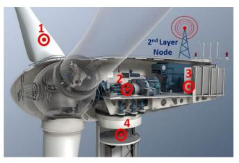
Figure 7. Possible third-level sensor (red circle) deployment inside the nacelle of a wind turbine.
