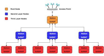
Figure 5. Hybrid tree-mesh network architecture.
