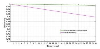
Figure 9. Comparison of the predicted reliability trend without redundancy and using a warm standby configuration.
