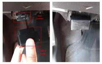
Figure 2. Communication interface between a typical OBD-II device and a vehicle.
