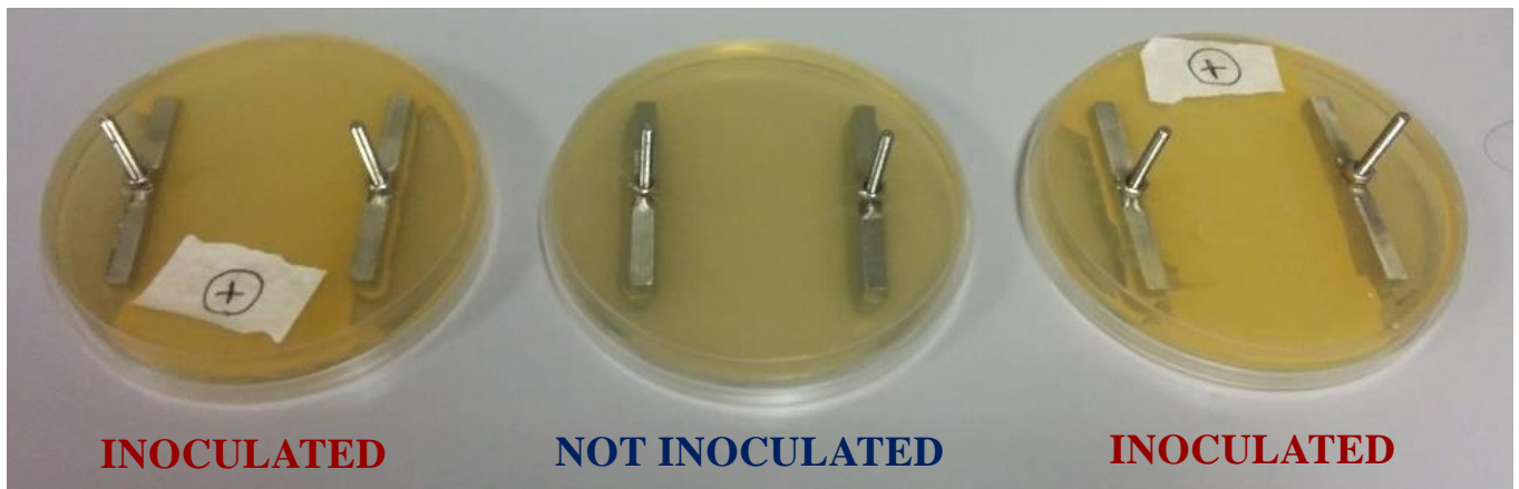
Figure 8. Petri dishes at the end of a preliminary test in which C_0 = 4.5 \cdot 10^8 CFU/ml.
