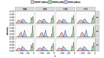
Figure 5. RS-related epdf for each TM and Codeword for Band 1 (2100  $\ensuremath{\mathsf{MHz}}\xspace).$
