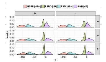
Figure 4. RS-related epdf for each TM and Codeword for Band 20 (800  $\ensuremath{\mathsf{MHz}}\xspace).$
