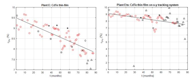
Figure 4. Estimated efficiency of the plants based on CdTe PV modules: E in fixed installation, E<sub>ts</sub> on an x-y tracking system (red circles); black squares: values after the adjustment of the monitoring system; black stars: values after module washing; black diamonds: values obtained by means of the capacitive load technique; black triangles: invalid data.
