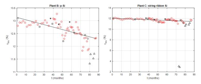
Figure 5. Estimated efficiency of the plants based on p-Si modules (left chart) and string ribbon Si modules (right chart) (red circles); black squares: values after adjustment of the monitoring system; black stars: values after module washing; black diamonds: values obtained by means of the capacitive load technique; black triangles: not valid data.
