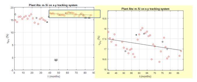
Figure 2. Estimated efficiency of plant A<sub>ts</sub> based on m-Si PV modules on an x-y tracking system (red circles); black squares: values after adjustment of the monitoring system; black stars: values after module washing; black diamonds: values obtained by means of the capacitive load technique; black triangles: invalid data.
