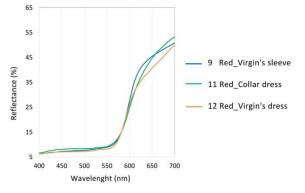
Figure 6. VIS-RS spectra of red colours. Identified pigment: 9, 11, and 12 - cinnabar.
