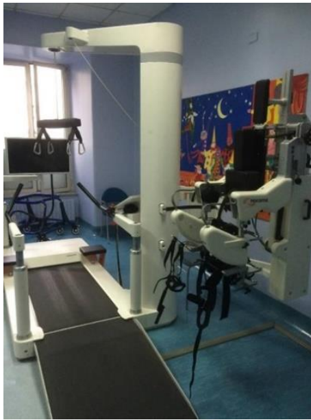
Figure 5. The driven gait orthosis Lokomat guides the legs of the subject walking on the treadmill. A body weight support system further facilitates the walking movements.
