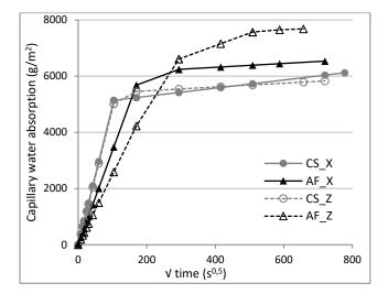
Figure 1. Capillary water absorption  $(g/m^2)$  vs. square root of the time  $(s^{0,5})$  along the two investigated directions (X and Z).
