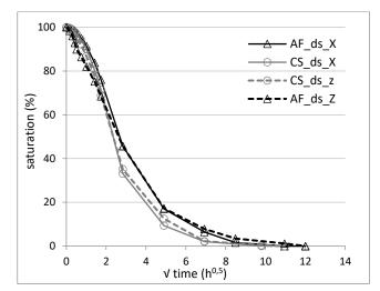
Figure 2. Water desorption curves. Saturation (%) vs. square root of the time  $(h^{0.5})$  along the two investigated directions (X and Z).
