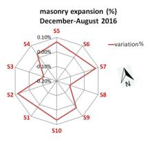
Figure 3. Variation (%) of opposite sides distances between 3D laser scanning surveys of August and December 2016.
