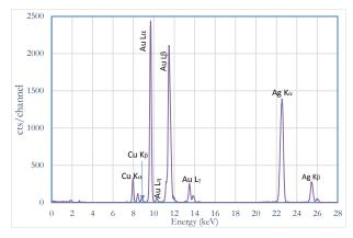
Figure 3. X-ray spectrum of an Au-Ag-Cu alloy, obtained with the equipment shown in Figure 2; the X-ray tube was working at 35 kV and 30  $\mu$ A. The X-ray peaks are, from left: Cu-K $_{\alpha}$  line (8 keV), Au-L $_{1}$  (8.5 keV), Cu-K $_{\beta}$  (8.9 keV), Au-L $_{\alpha}$  (9.7 keV), Au-L $_{\alpha}$  (10.3 keV), Au-L $_{\beta}$  (11. keV), Au-L $_{\gamma}$  (13. keV), Ag-K $_{\alpha}$  (22 keV), and Ag-K $_{\beta}$  (25 keV). Au X rays.
