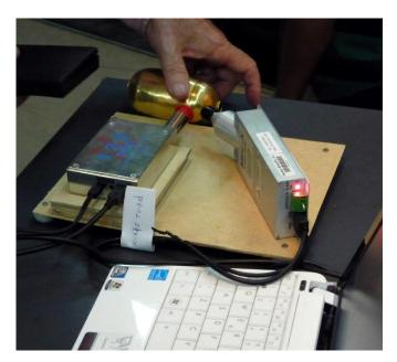
Figure 2. Energy-dispersive X-ray fluorescence portable equipment, composed of a Si-drift detector (on the right; 123 SDD: 450  $\mu m$  thickness, 7 mm² area, and 125 eV energy-resolution at 5.9 keV) and an Ag-anode X-ray tube (40 kV, 100  $\mu A$  maximum voltage and current) [10]. Electronics including bias supply and Multi-Channel Analyzer (MCA) are in the case of the detector; X-ray tube bias supply is in the case of the X-ray tube. A typical measurement takes 50–100 s.
